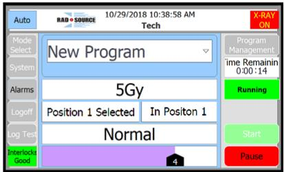
5) When the exposure is complete the buzzer will sound and the status indicator will change from "Running" to "Complete\*." Open the door, remove the product, and close the door.
