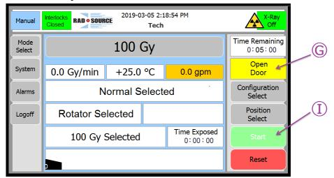
3) While the door is open the Interlocks Indicator's background will be Orange and it will display "Interlocks Open" (a). The yellow Instruction Box will display "Close Door" (a). The Start Button (b) will remain a light green.
