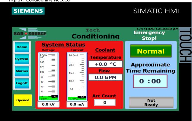
**NOTE:** The condition mode is set to 15 min, running down time before Automatic mode starting. (At least once every 24 hours) and 30 min on extended running down time if not running for 7 days.
