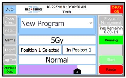
2) When the machine has been paused, you may either resume the cycle by pressing Resume\*, or cancel the cycle by pressing Stop\*
