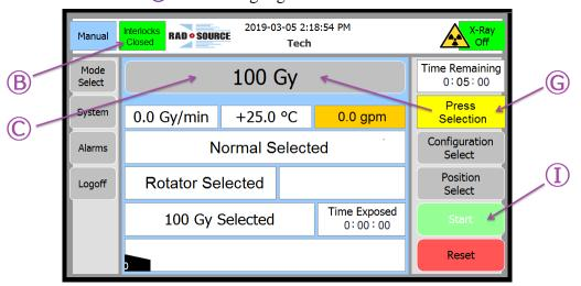
5) Select the correct configuration by touching the *Configuration Select* ① button to cycle through the available configurations. Touch the *Position Select* ① button to select the desired position. Press *Start* ① to begin the cycle.
