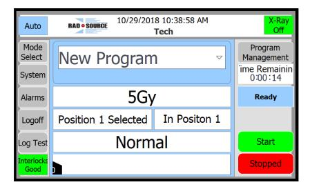
4) During X-ray generation a variety of buttons will turn white, indicating that they are unavailable for selection, a Progress Bar\* displaying the total Grays (Gy) produced will run from left to right across the bottom of the screen, the X-ray On indicator\* will flash, and the status indicator will display "Running."\*
