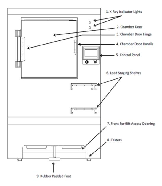
Fig.1: Front View of the RS 420
