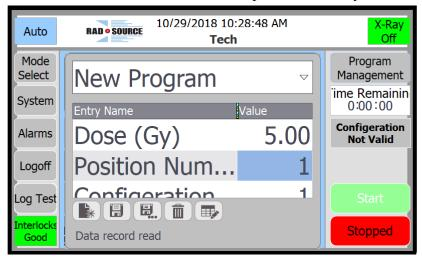
6) Press the Configuration Select button ① to cycle through the available configurations, then, enter the corresponding number into Value column next to Configuration
