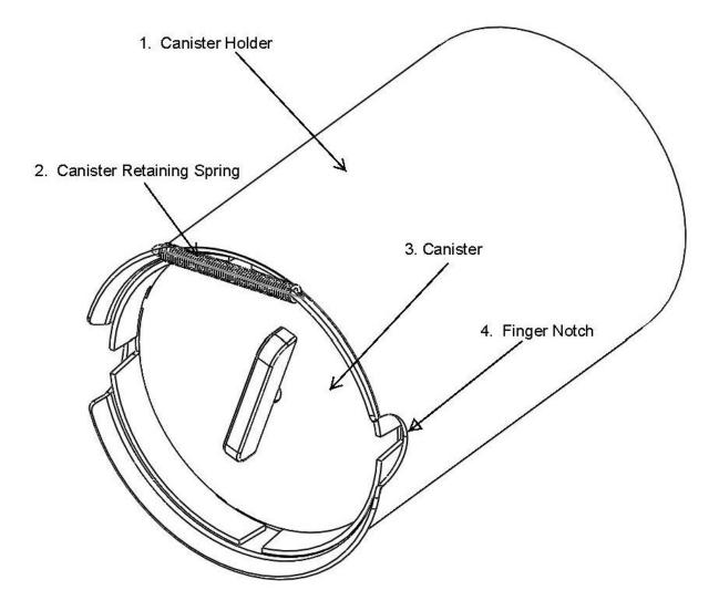
1. **Canister Holder** – This is attached to the rotation assembly within the Chamber and is used to hold the Canisters during irradiation. It is aluminum with a slight flare at its opening to allow the Canisters to be easily inserted.
