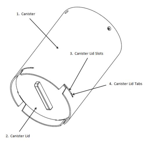
1. **Canister** – This is required for containing the products intended to be irradiated. The standard Canister is approximately 7" in diameter by approximately 6" in overall height. The Canister bottom is fixed in place and the removable lid has a handle.
