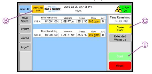
4) Unless some other interlock is open, once the door is closed the, Interlocks Indicator's background will become Green and it will display "Interlocks Closed" (B). The yellow Instruction Box will be replaced by as light blue System Status Box which will display "Ready" (G). The Start Button (I) will be a sold green indicating the system is ready to run "Warm Up"
