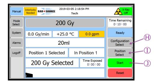
**NOTE:** The Time Remaining display will automatically adjust the cycle time according to the selections made.
